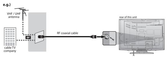
\*Once connections are completed, turn on the unit and begin initial setup.
